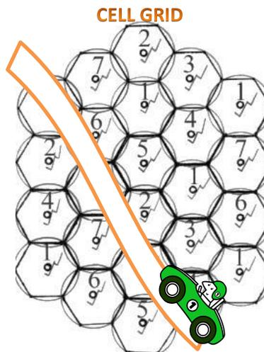
the design uses hexagon shapes to show each cell with an overlapping circle to show signal range from the base station. Seven cells in a cluster will make up a working system. Each cell in the cluster needs a separate frequency and must not share the same frequency in an adjacent cell. A cell-phone carrier typically gets 832 radio frequencies for the entire city system. In order to work, each cell will have from 56 to 168 voice channels available depending on the digital
