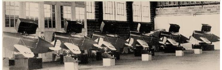
The ANT-18 became standard equipment to every military training school in the U. S. and its' allies introducing tens of thousands of fledgling pilots to the basics of instrument flight. During the war years, Link manufactured over 10,000 units turning out one every 45 minutes.
