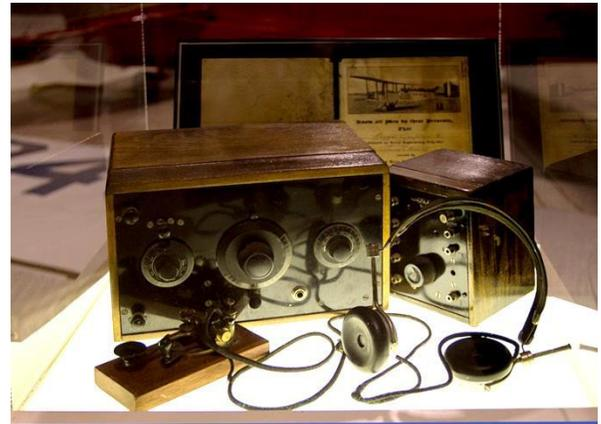
**Standard land line telegraph hand key & radio headset, with transmitter on display at Golden Wings Museum**
