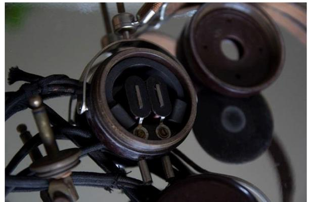
**Headset electronics receive signal at two electro magnets. When changes in signal amplitude are received a thin disk in the ear piece will vibrate producing the signal reproduction.**
