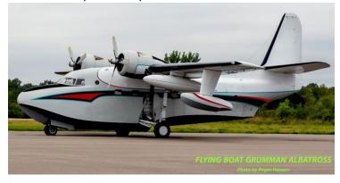
Flying boats, as the name suggests, have a fuselage or body with a bottom shaped like a boat's hull and is hydrodynamically shaped for efficiency in water operations. Typically, they have two small floats or pontoons at the wing tips to stabilize the plane when operating on water. Floatplanes are usually land based aircraft converted to Floatplanes by removing the wheels and attaching floats or pontoons.
