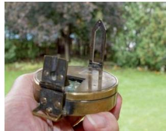
accurately called **Inclinometers** used for surveying and plotting building construction but were useful as a sighting tool for the early pioneering pilot. The disk would be aligned by viewing a distant object through the upright sighting frames. At the same time sighting through the magnifying glass would reveal what is called the **Azimuth** number corresponding to the direction being viewed.
