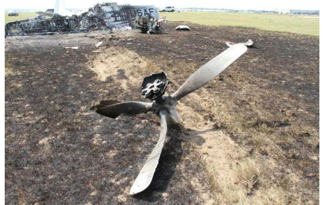
Here you can see how they propeller separated from the engine taking with it a portion of the gearcase housing and the planetary gear set.
